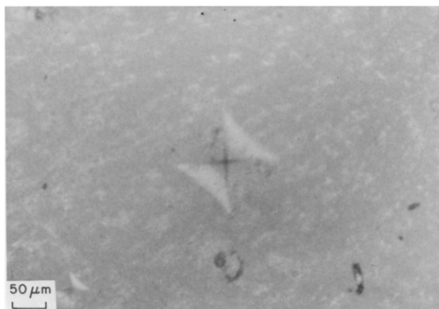
Figure 2 Photograph of the Vickers microindentation obtained with a load of 2 N and taken with a microscope objective of \times 20
